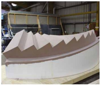
Cordek's project design team created an inverted 3D model of the staircases orientated to optimise the precasting process Cordek's project design team created an inverted 3D model of the staircases orientated to optimise the precasting process. This digital model was programmed into Cordek's five-axis CNC router to manufacture an accurate pattern for the staircase.
