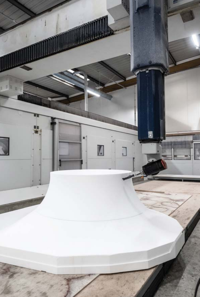
A five-axis router used in the manufacture of an EPS 'dome' former.
