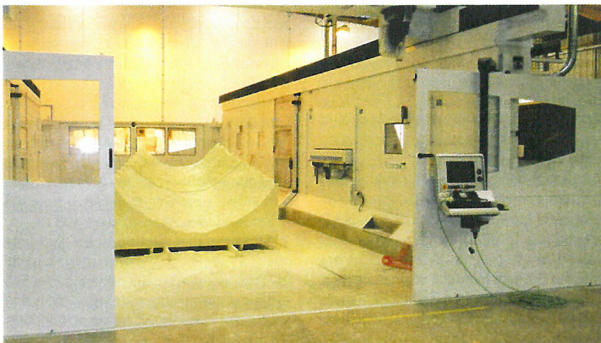
Figure 5 below right: Moulds being prepared for epoxy seal coat.
