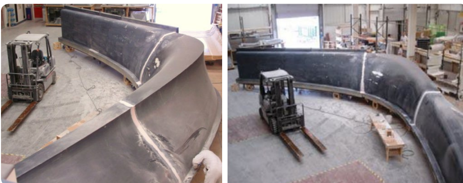
Figure 5a and b: Complete pattern for left side of the 10m dice tower being finished ready for mould laminating.
